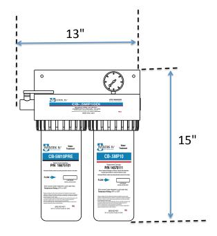
All carbon block cartridges should be changed out every six months or when there is a reduction in water pressure. Filter life depends greatly upon the quality of water. This product is for commercial use only and must be installed and maintained according to manufacturers guidelines www.systemsiv.com or the warranty can be voided.
